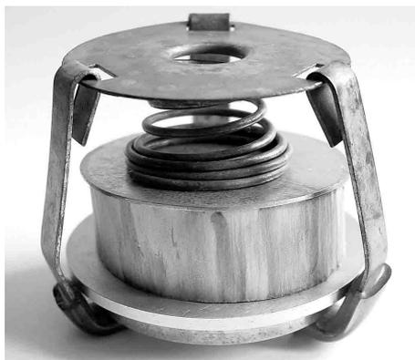
Fig. 2. Wood sample in the grip with the pressing elastic element
