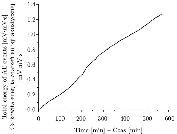
Fig. 12. Total energy emitted by birch sample during drying process
