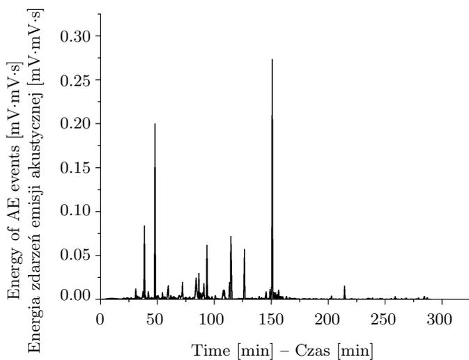
Fig. 4. Energy of AE signals generated in oak sample during drying
