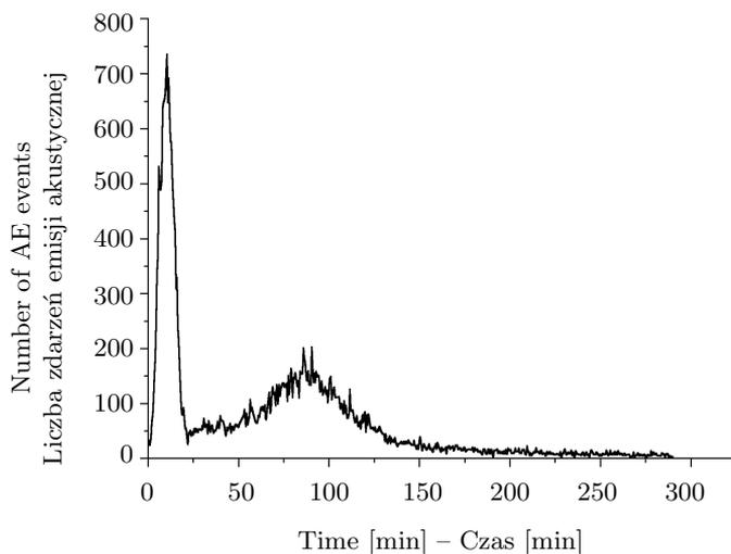
Fig. 3. Exemplary plot of AE signals emitted during drying of oak samples
