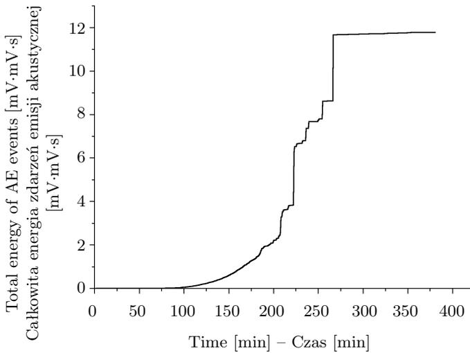
Fig. 9. Total energy emitted by pinewood sample during drying process
