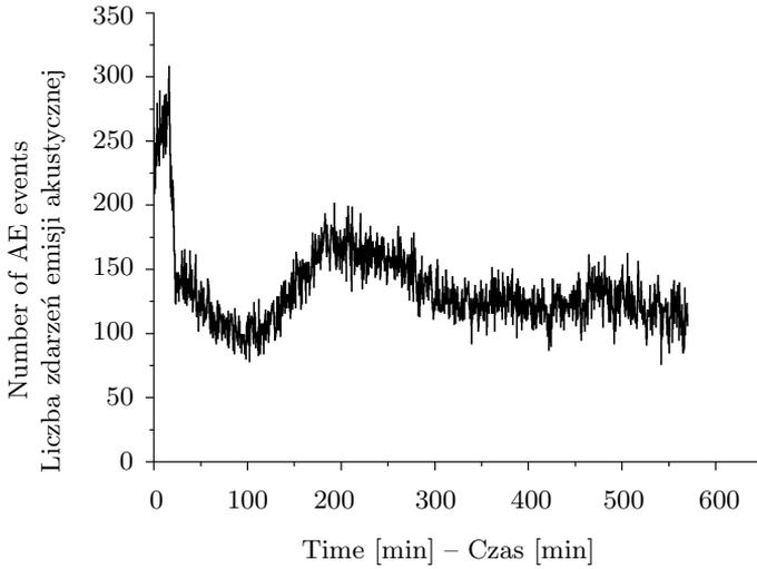
Fig. 11. Exemplary plot of AE signals emitted during drying of the birch samples
