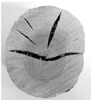
Fig. 6. Appearance of macrocracks in oak sample arisen after the stress reverse
