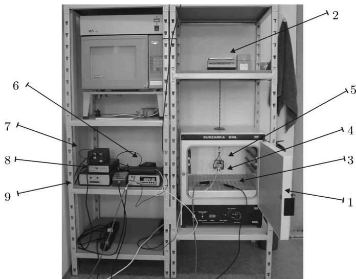
Fig. 1. Measuring set up for acoustic emission (AE): 1 – chamber drier, 2 – balance, 3 – temperature and humidity sensors, 4 – piezoelectric transducer, 5 – wood sample, 6 – AE detector, 7 – amplifier, 8 – conversion of AE signals, 9 – GPID card
