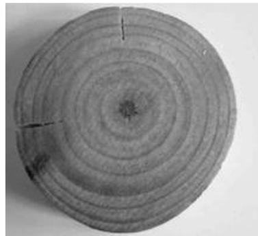
Fig. 10. Appearance of macrocracks in pinewood sample arisen during drying
