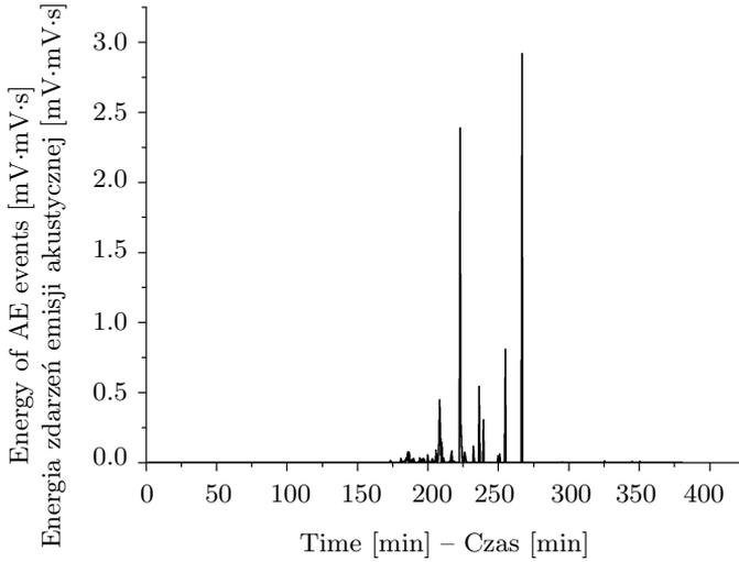
Fig. 8. Energy of AE events generated by pine during drying
