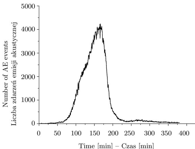
Fig. 7. Exemplary plot of AE signals emitted during drying of the pinewood samples
