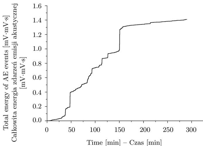
Fig. 5. Total energy of AE signals emitted by oak wood sample during drying
