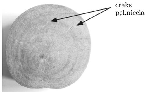
Fig. 13. Appearance of macrocracks in birch sample arising during drying
