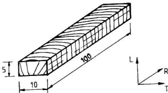
Fig. 2. Samples shape and dimensions
