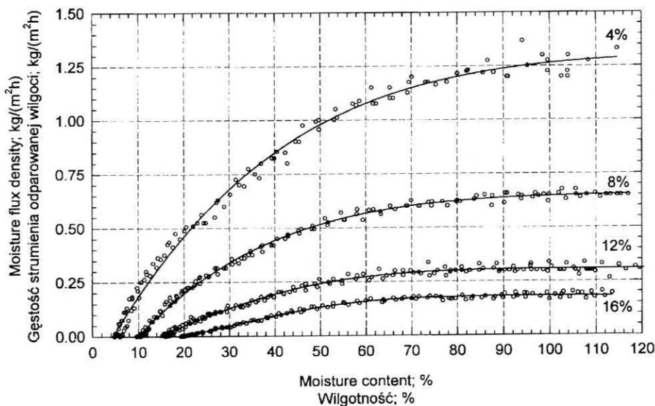
Fig. 5. The influence of equilibrium moisture content on moisture evaporation rate, temperature  $t = 60^\circ\text{C}$
