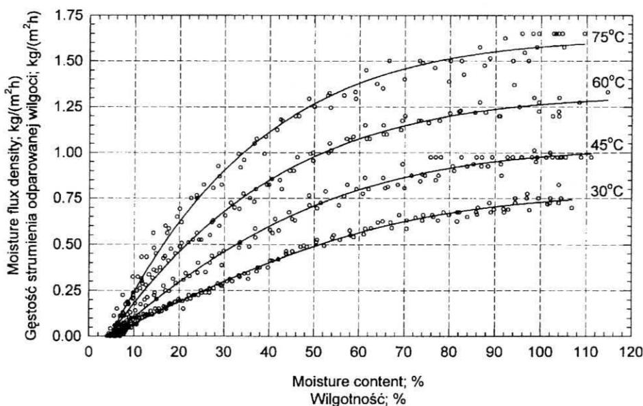
Fig. 6. The influence of temperature on moisture evaporation rate, equilibrium moisture content  $EMC = 4\%$
