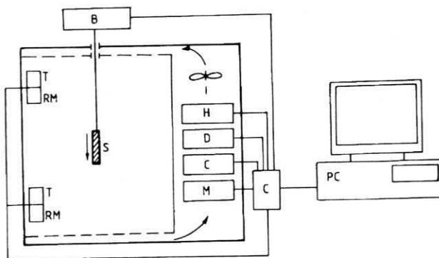
Fig. 1. Scheme of experimental stand: S - sample, B - balance, T - temperature sensor, RH - relative humidity sensor, H - heater, D - drying unit, C - cooler, M - moistening unit, C - a/d converter, PC - personal computer
