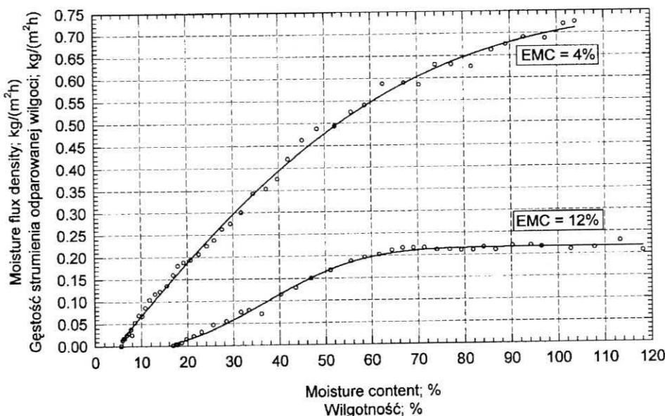
Fig. 4. The flux density of evaporated moisture vs. moisture content ( $t = 30^\circ\text{C}$ ,  $\text{EMC} = 12\%$  and  $\text{EMC} = 4\%$ )
