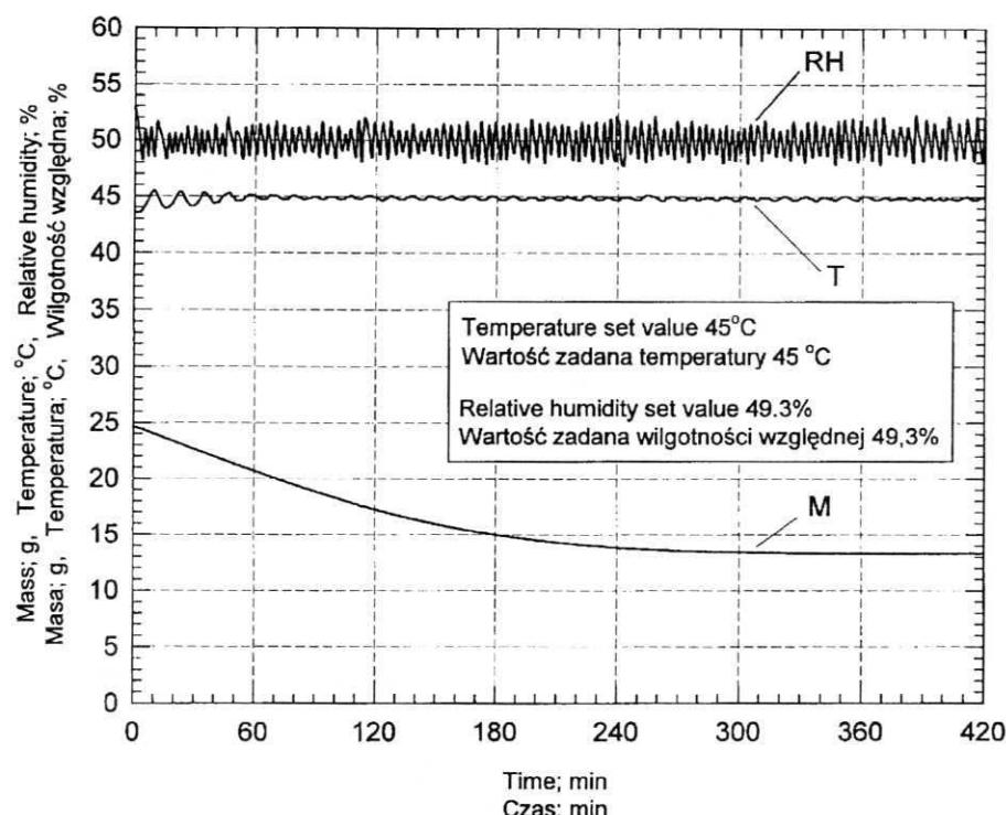
Fig. 3. Changes of samples mass and air parameters during a drying process ( $t = 45^{\circ}\text{C}$ ,  $\text{EMC} = 8\%$ )
