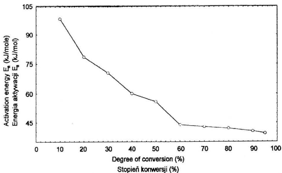
Fig. 6. Changes of activation energy vs. degree of conversion for degradation process of Jowatherm 280 70 adhesive
