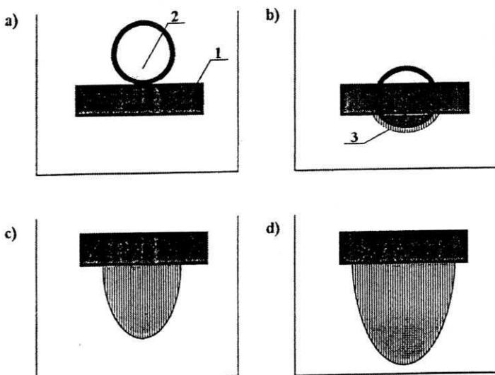
Fig. 1. Scheme of the stages at determination of the softening temperatures HM adhesives by ring-ball method
