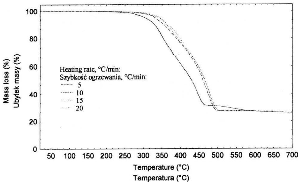
Fig. 3. TG thermograms for Jowatherm 227 20 adhesive at selected heating rate
