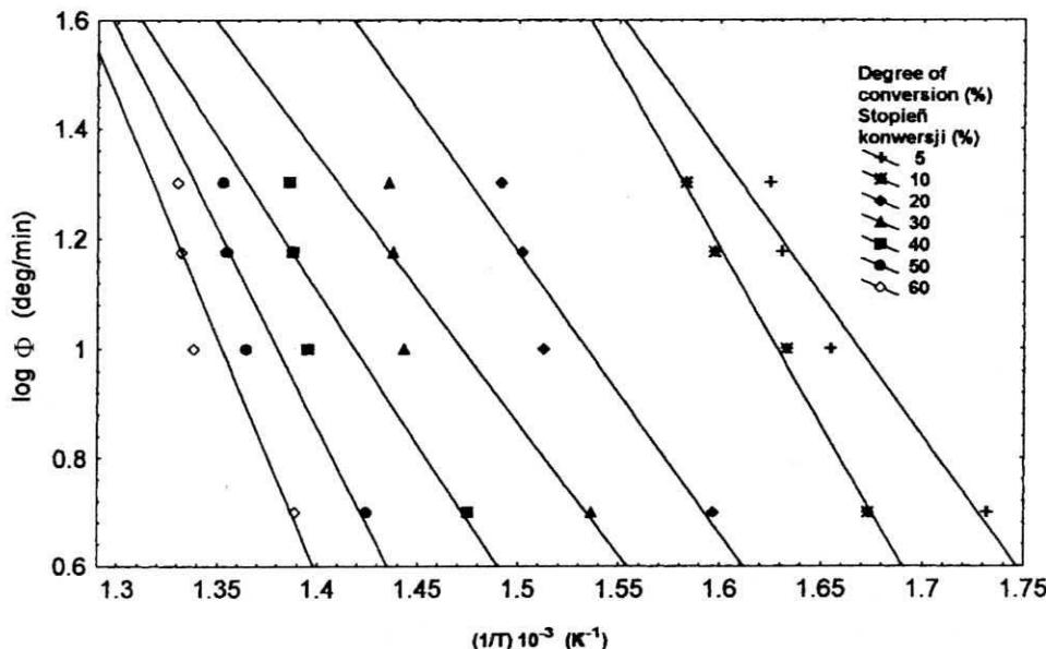
Fig. 4. Plot  $\log(\Phi)$  vs.  $(1/T)$  for thermal degradation process of Jowatherm 227 20 adhesive
