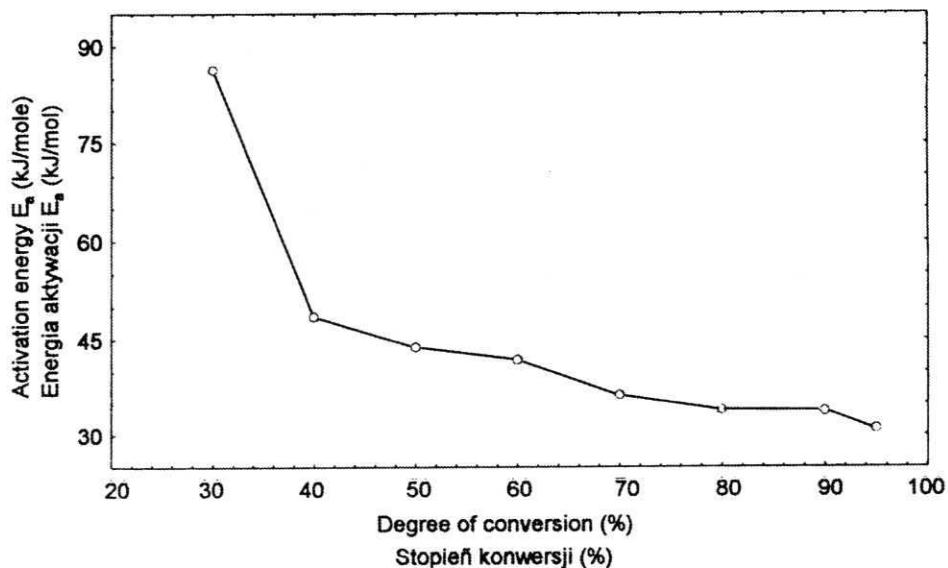
Fig. 5. Changes of activation energy vs. degree of conversion for degradation process of Jowatherm 227 20 adhesive
