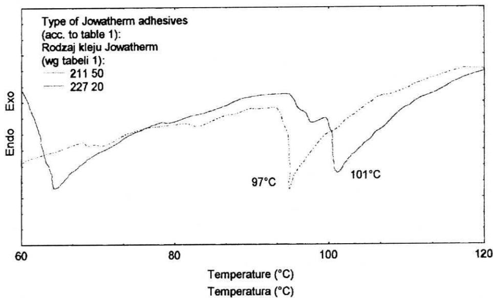
Fig. 2. DTA thermograms for selected Jowatherm adhesives at heating rate 5°C/min
