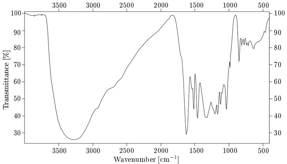
Fig. 6. IR spectrum of the dry residue of substances from the merbau wood soluble in hot water
