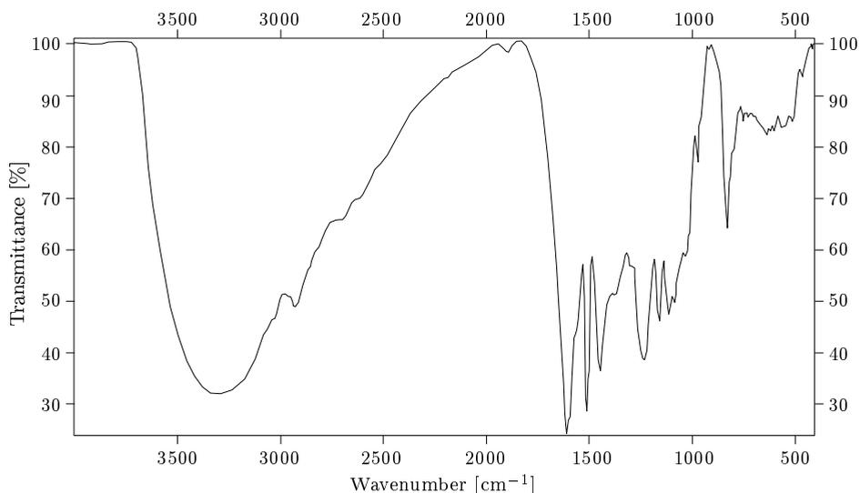
Fig. 4. IR spectrum of the dry residue of substances from the doussie wood soluble in hot water
