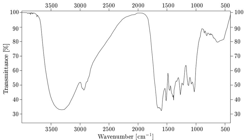
Fig. 8. IR spectrum of the dry residue of substances from the sapwood soluble in hot water
