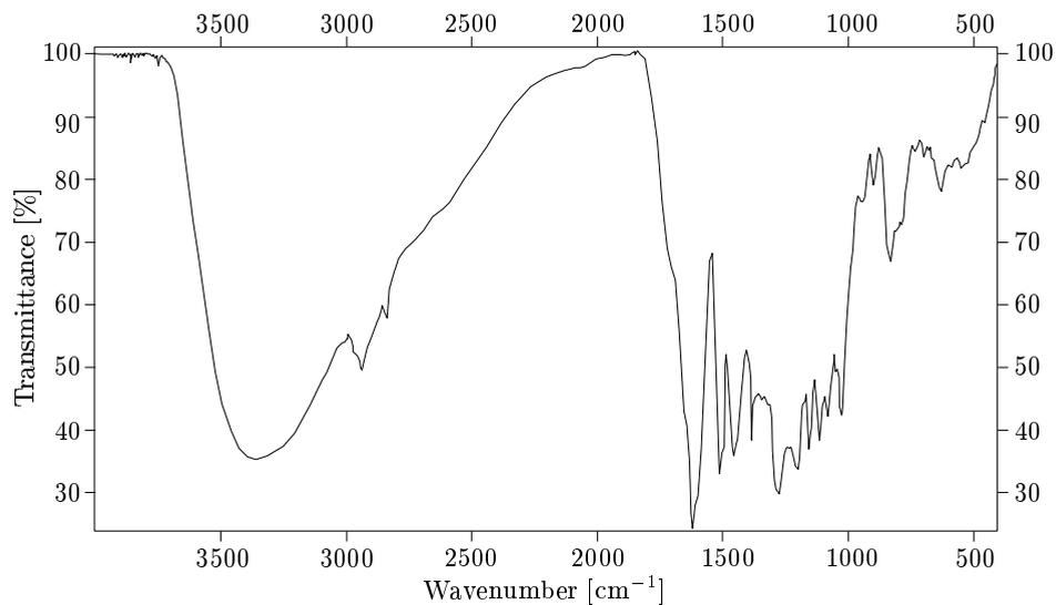
Fig. 7. IR spectrum of the dry residue of substances from the padouk heartwood soluble in hot water
