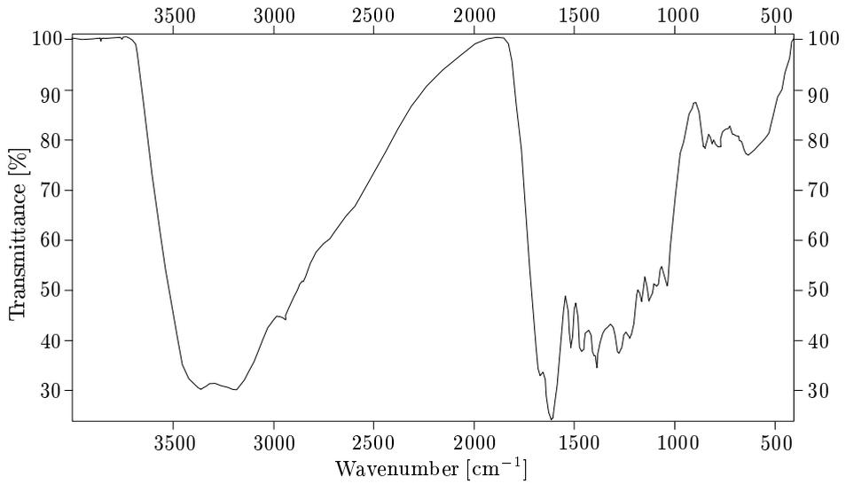
Fig. 5. IR spectrum of the dry residue of substances from the wenge wood soluble in hot water
