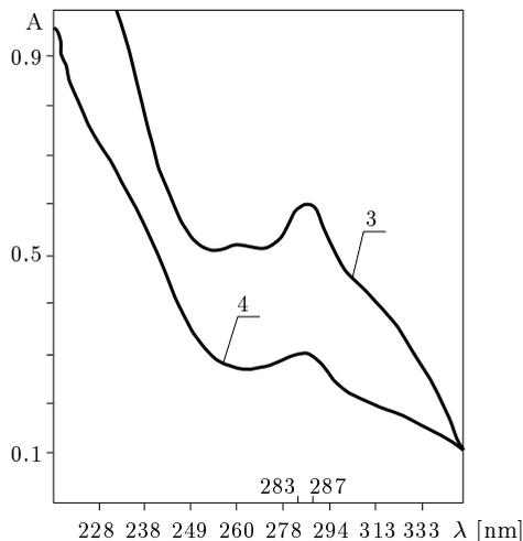
Fig. 3. Course of the UV spectrum of substances from the padouk wood soluble in hot water: 3 – heartwood (dilution 1:20), 4 – softwood (dilution 1:20)
