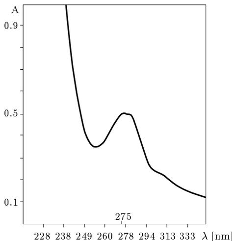
Fig. 1. Course of the UV spectrum of substances from the doussie wood soluble in hot water (dilution: 1:20)
