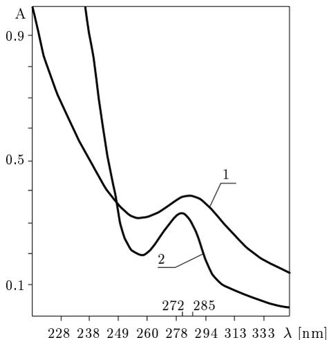
Fig. 2. Course of the UV spectrum of substances from wood soluble in cold water: 1 – the wenge wood (dilution 1:4), 2 – the merbau wood (dilution 1:10)
