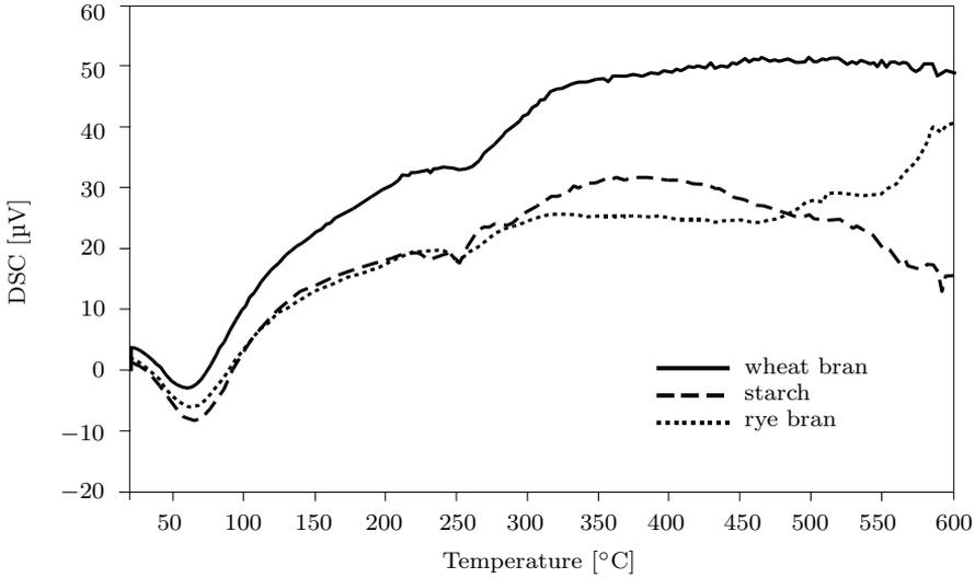
Fig. 3. DSC curves of wheat bran, starch, and rye bran
