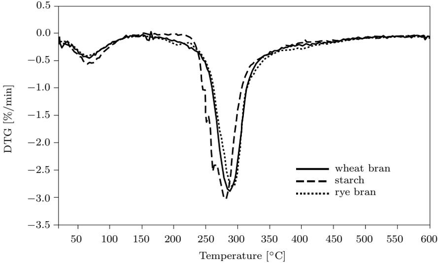
Fig. 1. DTG curves of wheat bran, starch and rye bran
